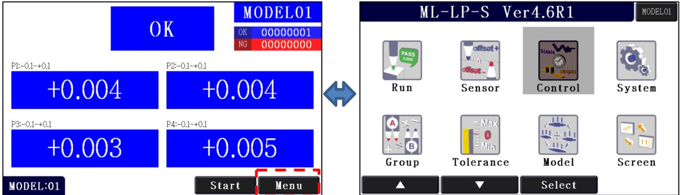
If the 'Menu' on the screen or the mode button(■) is pressed, the main menu is appeared. The main menu is reached in the any other menu by pressing the Mode button(■) several times. The menus shown on the screen can be entered by touching the screen or moving the cursor by Up(▲) /Down(▼) buttons and pressing Select(▶) button on it.
